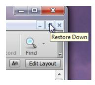
In order for the compiled WinAutomation job to find menu items within the FileMaker user interface, the database window should not be maximized.
