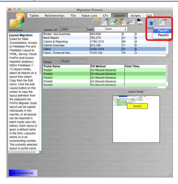
On the Layouts tab, click the Create All Layouts in FileMaker button. The Pass#1 pop-up menu should be selected under the Create All Layouts in FileMaker button.
