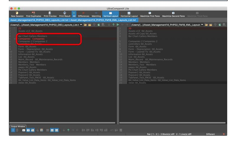
Line #1 displays a difference due to the different count of layouts. But Line#5 is where the difference exists for the list of layouts. The layout named Companies (using a TO with the same name) shown on the left side as an extra layout which is the missing layout from the FileMaker database XML export shown on the right side.
