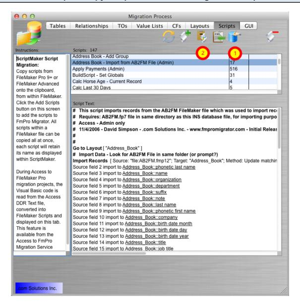
Use the [1] Create All Scripts in FileMaker batch processing button to create each script one at a time in batch processing mode (macOS only).
